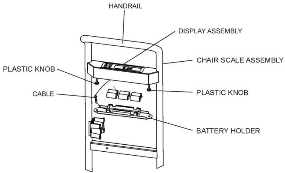
**Figure 4. Replacing Batteries**
